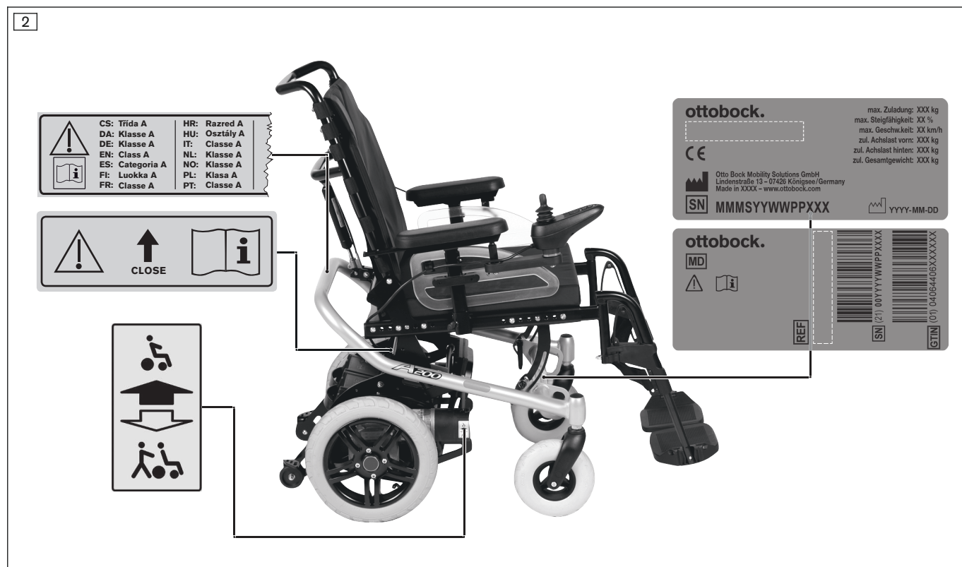
Warning signs and nameplates on the power wheelchair
